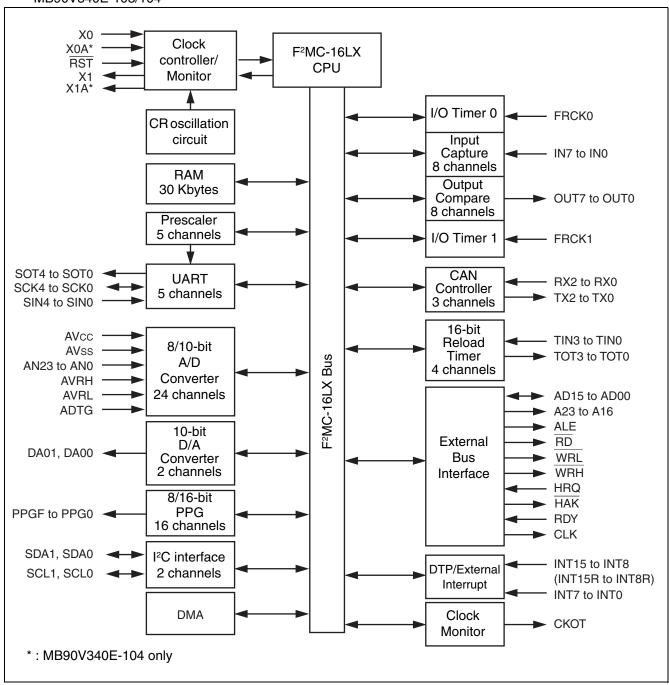
MB90F352E (S), MB90F352TE (S), MB90F351E (S), MB90F351TE (S), MB90352E (S), MB90352TE (S), MB90351E (S), MB90351TE (S)
